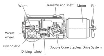
Friction adjustment mechanism
