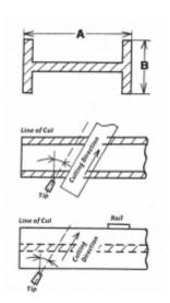
The **Mini-Mantis II** provides high-precision diagonal cuts that are clean and sharp. Two motors drives the torch for both web and flange cutting. No need to turn and mark the workpiece.
