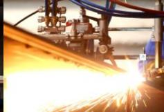
Chamfering (1:4 ratio bevelling) using single torch
