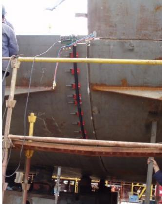
Welding preparation performed with 2D rail
